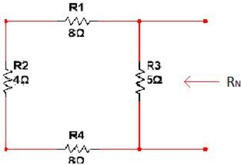
$$R_N = (4 + 8 + 8)\Omega // 5\Omega = 30\Omega // 5\Omega = \frac{(20\Omega)(5\Omega)}{20\Omega + 5\Omega} = \frac{100\Omega}{25\Omega} = 4\Omega$$
